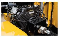
**35 HP (26 kW) GAS ENGINE.** The BC900xL is equipped with a Briggs & Stratton Vanguard gas engine, providing high torque in a compact and lightweight size to process branches and material up to 9" (22.9 cm) in diameter.
