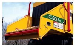
**OPERATOR SAFETY.** Combined with the patented bottom feed stop bar is the 4-position upper feed control bar with dual stop positions and forward/reverse feed positions. Mounted over the feed table, it enables the operator to stop the feed rollers and select forward or reverse operations. Dual reset/hold-to-run buttons allow the operator to readily reset the bottom feed stop bar.
